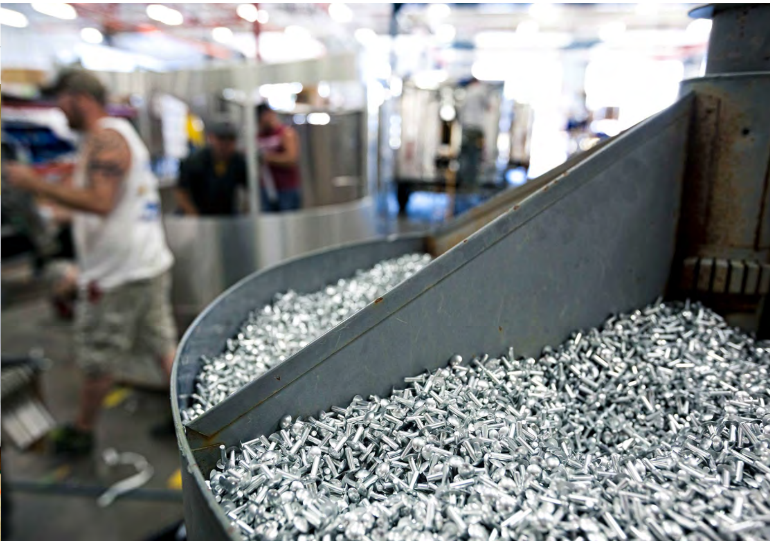
Opposite: The riveting process can be hard on workers' bodies, and normally entails two people. Above: Rivets must be reliably and evenly driven with no marring of the airplane skin, or else they must be drilled out, deburred, and redone.
