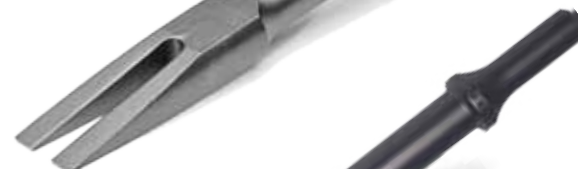
HET 159-A .498 Shank Slim Fork Chisel 8" O.A.L. With 30° Bend Made for narrow-spaced spot welds.
