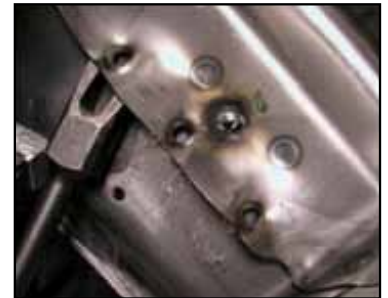
HET 97-8 Fork Expansion Chisel separating layers of metal, popping the weld nuggets.
