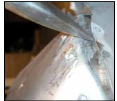
HET 26-1 Single Tine Expansion Chisel separating layers of metal, popping the weld nuggets.
