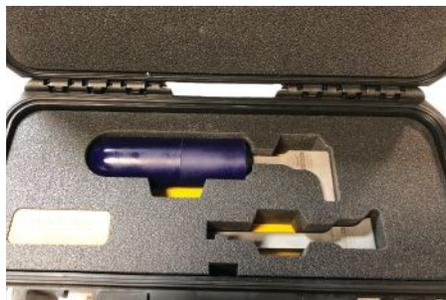
Because bucking bars can be required in potentially thousands of different shapes and sizes to suit specific aerospace applications, customization of the modular bar with interchangeable end effectors can also allow operators to reach a wide variety of difficult rivets.
