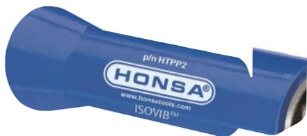
The advanced bucking bar, which was developed in collaboration with Richard Borcicky's expertise in safety and ergonomics, provides three levels of vibration reduction, including a wave spring, tungsten inserts, and a cushioned palm pad. Compared to traditional bucking bars, this reduces vibration up to 50%.
