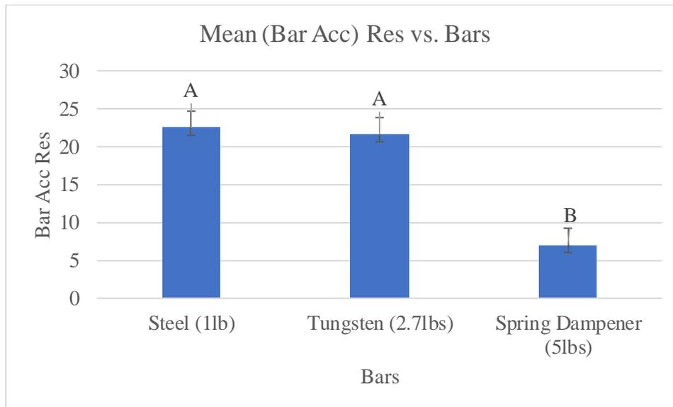
Figure 47. Mean Bar Acc Resultant vs. Bucking Bar
