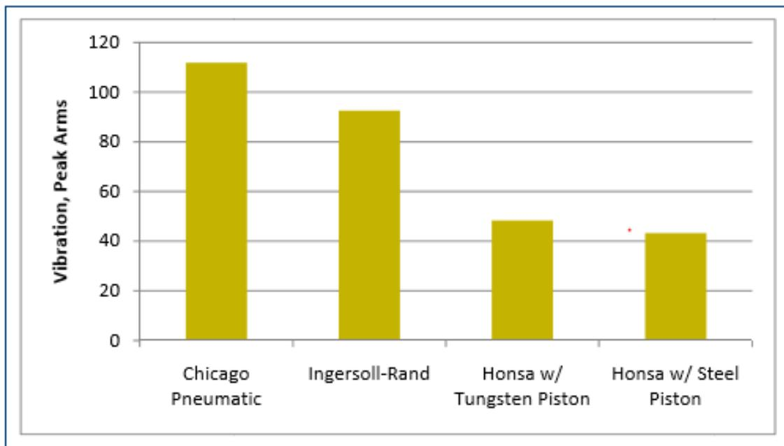
Figure 3. Peak Vibration (m/s<sup>2</sup>) Transmitted to the Operator Hand and Arm (HumanTech, Inc., 2010)
