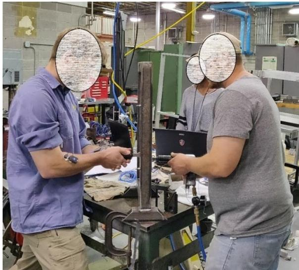
Figure 13. Experimental Trial with Rivet Gun Handle Grip in Vertical Position
