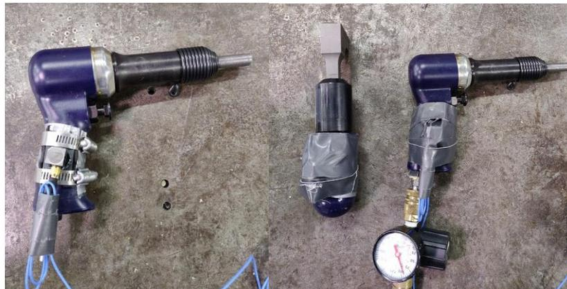
Figure 9. Triaxial Accelerometer Mounting on Bucking Bar and Rivet Gun
