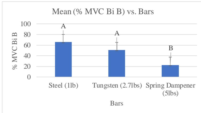
Figure 53. Mean %MVC Bi B vs. Bucking Bar
