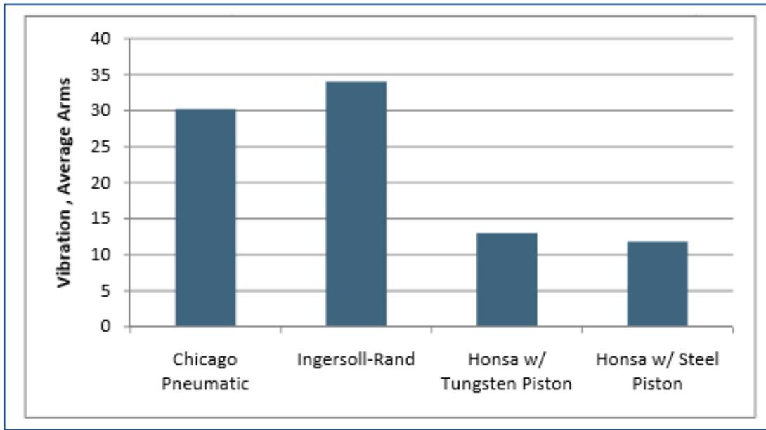
Figure 4. Average Vibration (m/s<sup>2</sup>) Transmitted to the Operator Hand and Arm (HumanTech, Inc., 2010)
