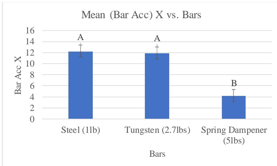
Figure 41. Mean Bar Acc X vs. Bucking Bar
