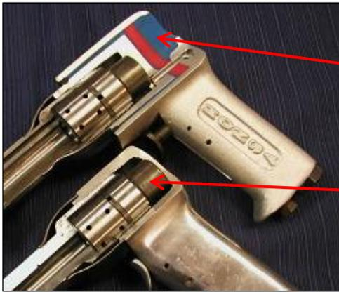
Honsa's Ergonomic Vibration Damping System. Note how this proprietary technology "isolates" the barrel and piston from the tool's grip, significantly reducing the transmission of damaging vibration to the operator's hands. And with no moving parts to break down or wear out, HONSA Low Vibration will last for the life of the tool. NO MAINTENANCE REQUIRED!
