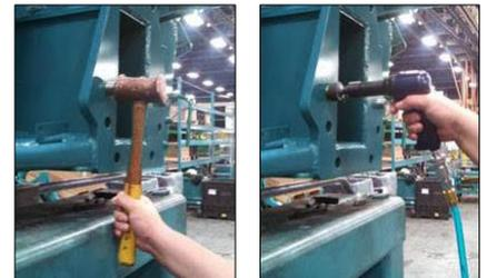
Here, an 8 lb. hammer is swung to drive 6 rods at 12 seconds per rod, or 72 seconds to complete the disassembly. The Honsa solution drives each rod in 2.75 seconds, or in less than 1/4 of the time.
